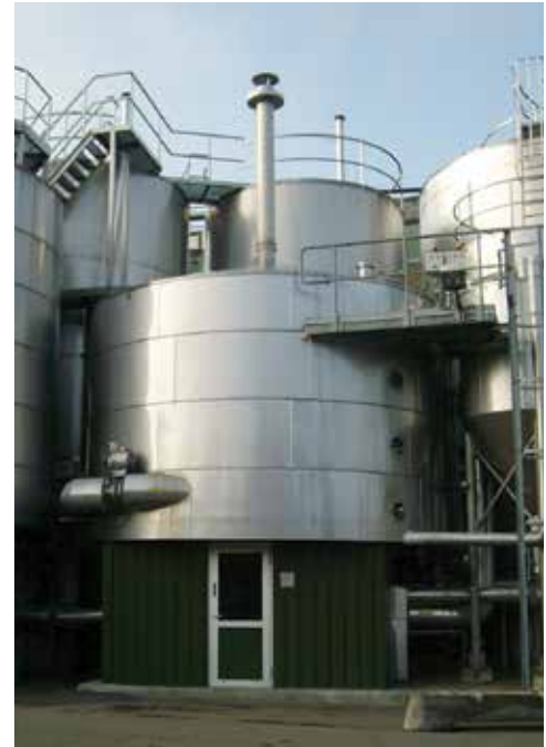
The whirlpool, where solid materials are separated out from the wort prior to fermentation.
