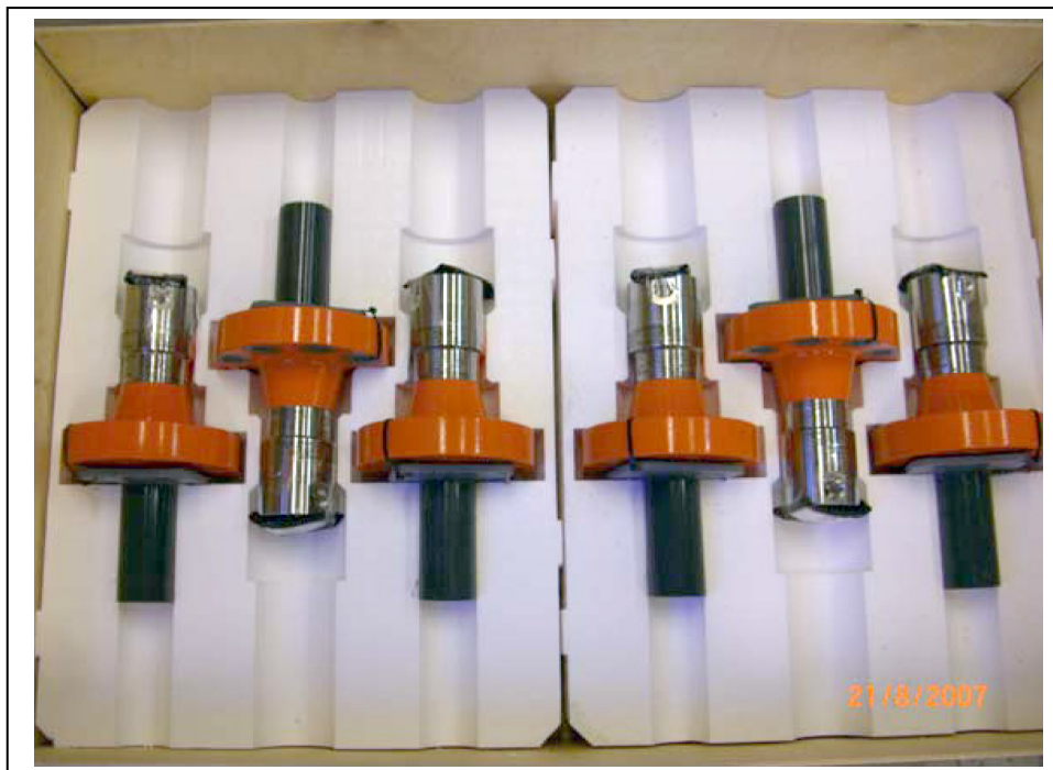
7.8.2 Typical packing of 6-off sensors within the Crate in 6.8.1
