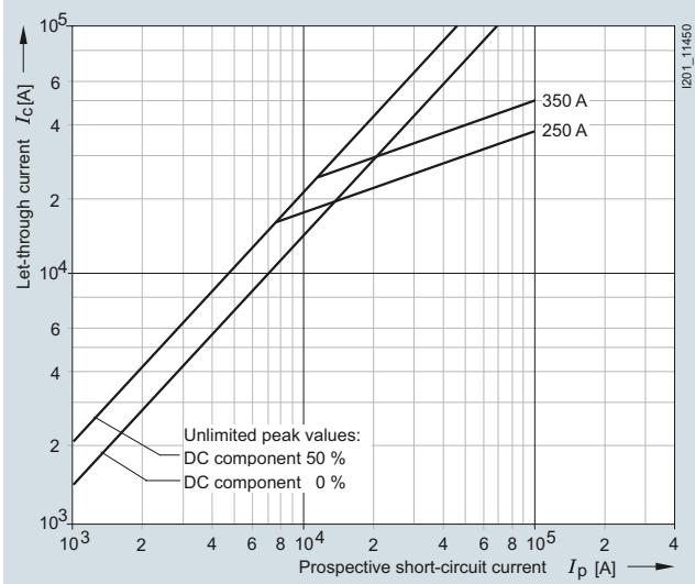
**Correction factor  $k_A$  for breaking  $I^2t$  value**
