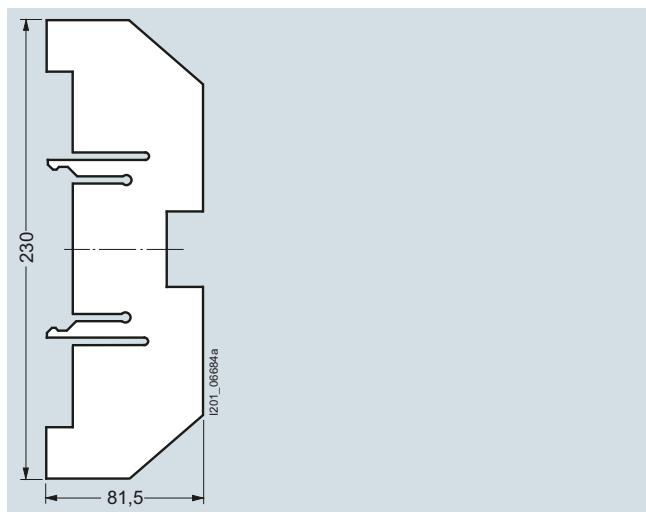
For LV HRC bus-mounting bases in tandem design
