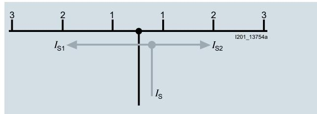
The sum of the output current per branch must not be greater than the busbar current  $I_{S1,2}$ /phase.
