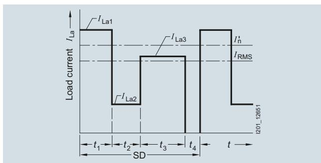
$$I_{\text{rms}} = \sqrt{\sum_{k=1}^n I_{Lak}^2 \times t_k} / SD$$
