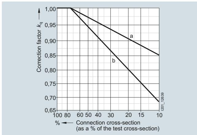
a = Reduction of cross-section of one connection
