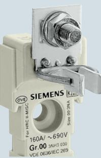
Flat terminals with screws are suitable for connecting busbars or cable lugs. They have a torsion-proof screw connection with shim, spring washer and nut. When tightening the nut, always ensure compliance with the specified torque due to the considerable leverage effect.
