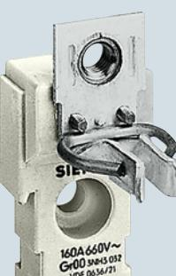
With the flat terminal with nut, terminal lug of the nut is torsion-proof. When tightening the nut, the torque must be observed because of the considerable leverage effect.
