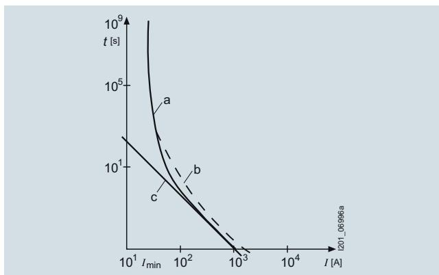
General representation of the time/current characteristic curve of a fuse link of operational class gG/gG
