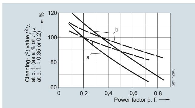
Breaking  $I^2t$  value  $I^2t_a$  of SITOR fuse links dependent on the power factor p.f.
