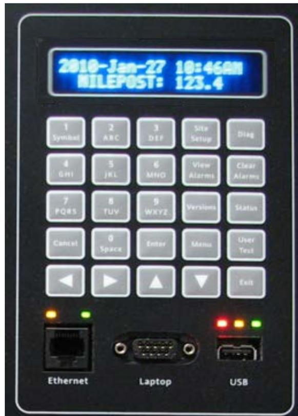
Figure 5-1 Local User Interface Display and Keypad
