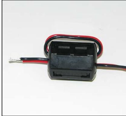
**Figure 3-7 EMI Filter Installed**
