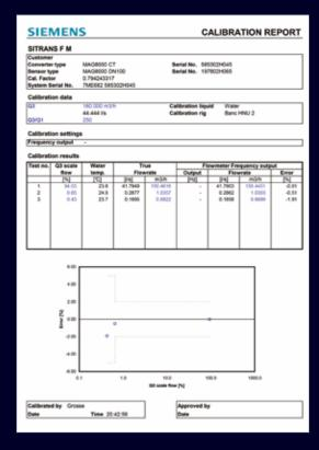
A calibration certificate is supplied with every water meter, and all calibration data is stored in the instrument.
