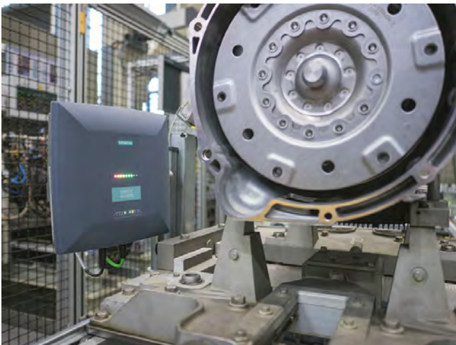
Figure 1. RFID systems are suitable for permanent electronic marking to identify and track products such as this vehicle transmission throughout its manufacture.
