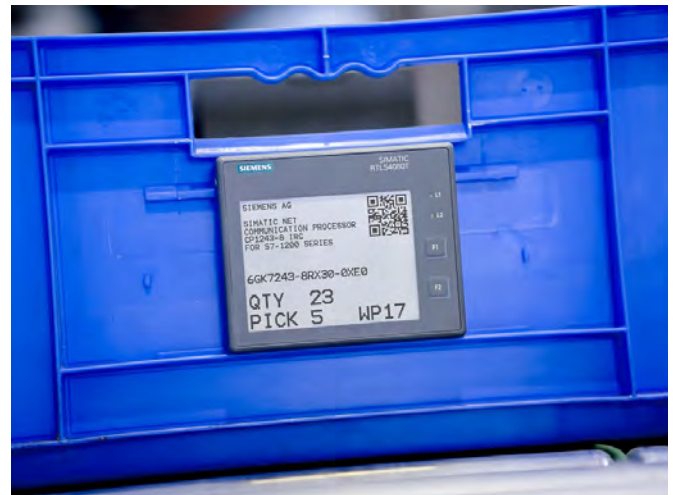
Figure 2. Through the SIMATIC RTLS data channel, it is possible to display data derived from the actual position and status of material containers.
