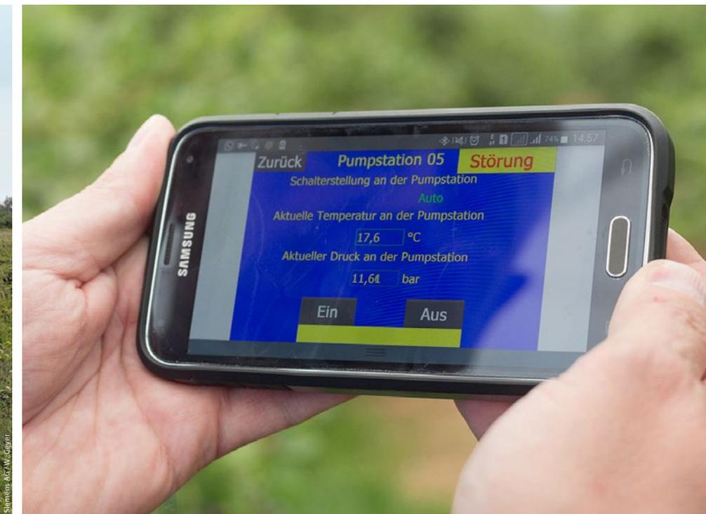
Thanks to the Smart Server option, personnel can switch the units on and off as well as control and monitor the pressure and temperature at each pumping station – even from a smartphone
