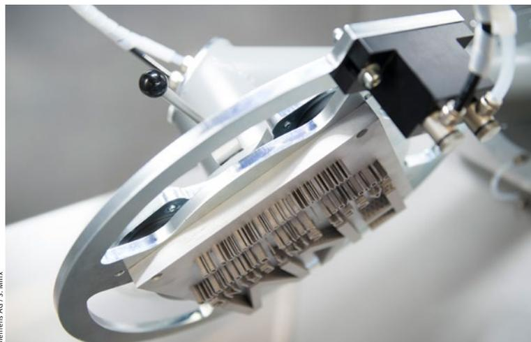
LOGO! 8 controls the swivel arm with a turntable onto which the component and platform are clamped
