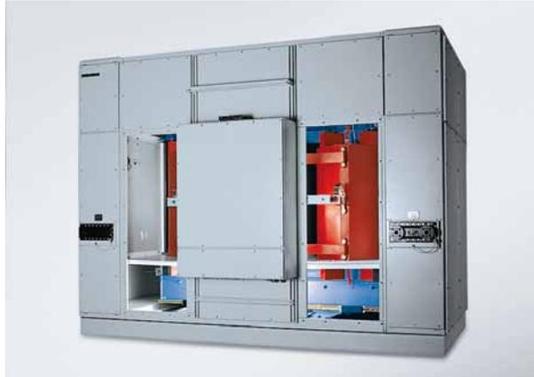
For the use in the Priobskoye oil field in Western Siberia: 7.5-MVA static converter transformers in double-tier design,  $35 \pm 2 \times 2.5\%/2 \times 2.2$  kV. Designed for ambient temperatures down to  $-55^{\circ}\text{C}$ . Transformer certification conforms to the Ghost standard. They were set up on a platform supported by a pile foundation.
