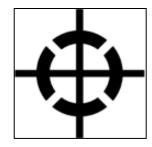
Fig. 19: Symbol for center of gravity
