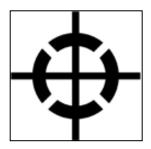
Fig. 168: Symbol for center of gravity
