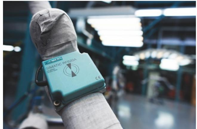
Four small RF620A antennas are installed on each gate in order to detect sills labeled on different positions (top/bottom).
