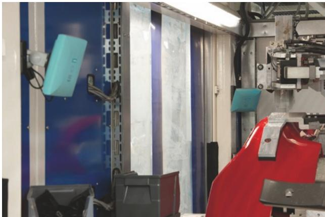
Also in the robotized punching, the parts are detected via RFID, relevant worksteps are initiated and absolved steps are indicated via the unique identification number (UID).
