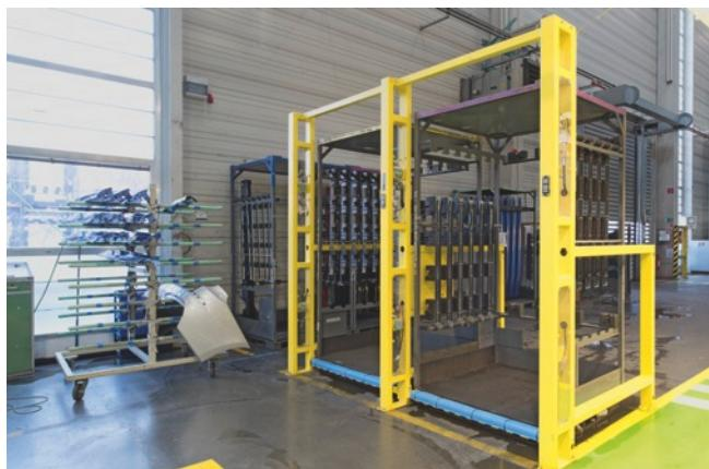
On so-called "sill gates", two antennas are connected to a reader via a splitter for space and cost reasons. Two antennas each detect the labels attached to the sills' top or bottom.
