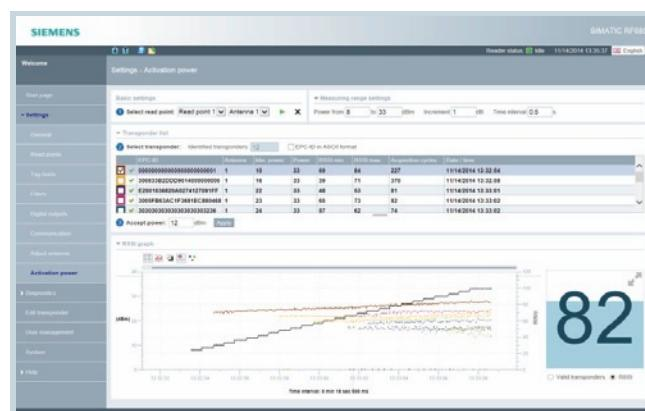
Easy handling via web browser: In the "Activation Power" menu of the reader's web interface, the parameters for a specific target transponder can be determined and parameterized without additional software.
