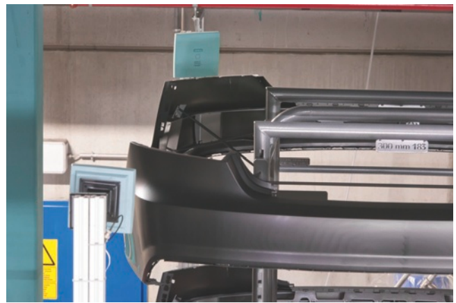
Based on the RFID labels, the system also checks the bumpers' positions on the paint skids, which helps to prevent damage to painting robots and parts.
