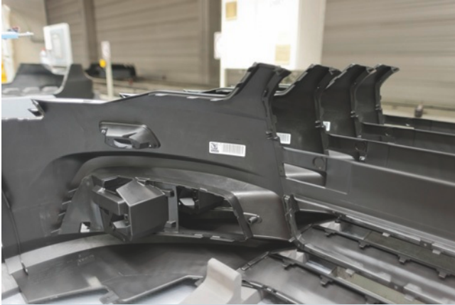
Using SIMATIC RF630L labels, Faurecia Automotive Exteriors traces injection-molded bumpers on their way through the process, provides the parts with quality features and detects these in the ERP system.
