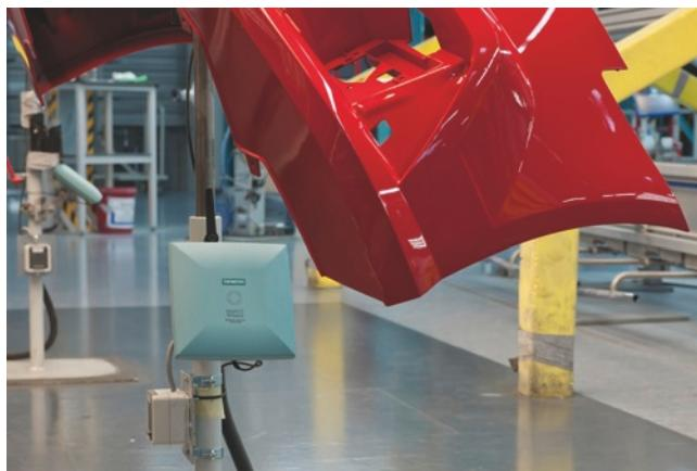
Instead of via handheld scanners, the parts are automatically detected during visual inspection in a contactless manner by means of RFID antennas (RF620A/RF640A) and the corresponding test screens are visualized.
