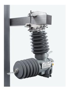
By eliminating regular maintenance and utilising line voltage as power supply, the new modular auto-recloser addresses common problems of obsolete hydraulic reclosers. The compact recloser is fully rated for voltage systems up to 27kV and features a complete insulated housing that covers all live parts. The lightweight device permits easy installation and fast commissioning, plus the ability for wireless firmware and configuration updates.
