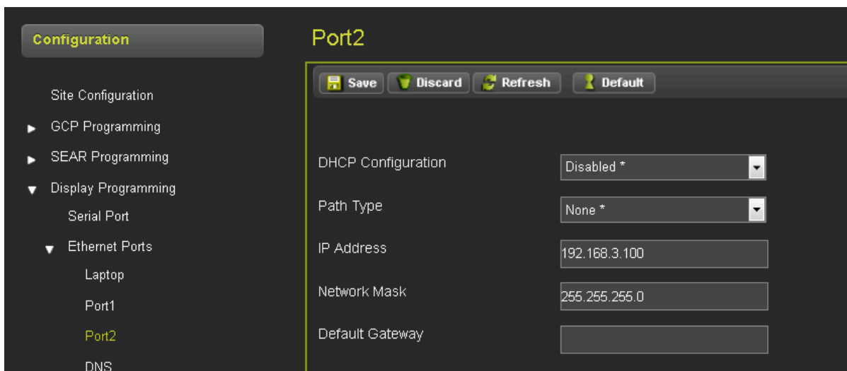
Figure 3-124: Display Programming Port 2 Ethernet Port
