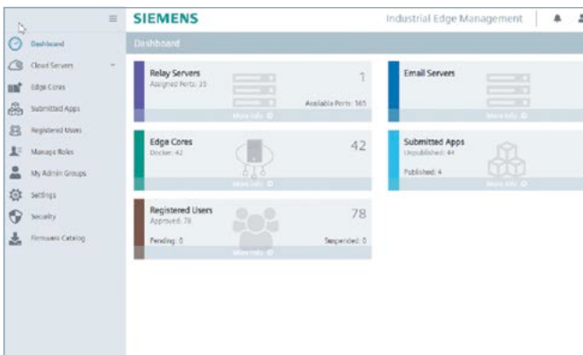
Administrator view for centrally monitoring globally registered devices, available and installed applications, and registered users in the system
