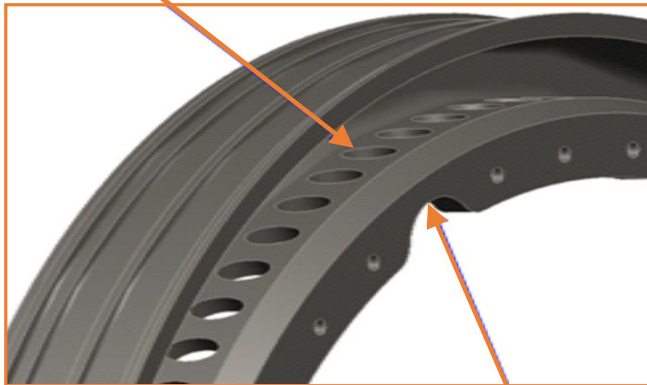
Slots to clear TD1 cooling holes
