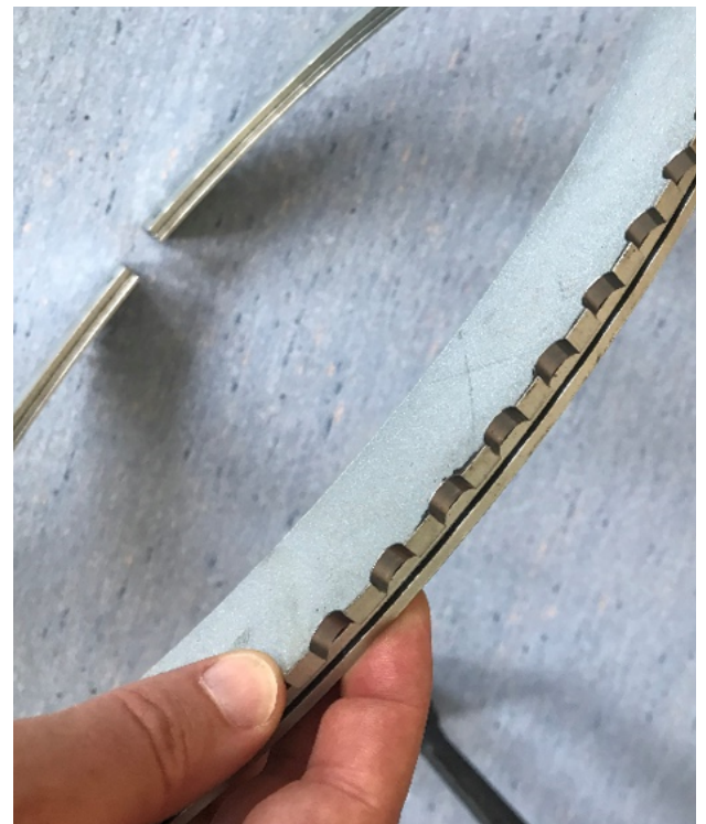
Fig. 8: Sound absorber variant for metro applications (tread brake).
