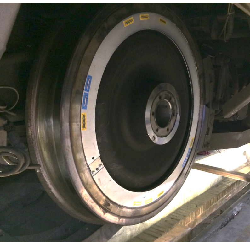
Fig. 9: Testing the sound absorber in high-speed operation (Velaro Novo) to reduce rolling noise.
