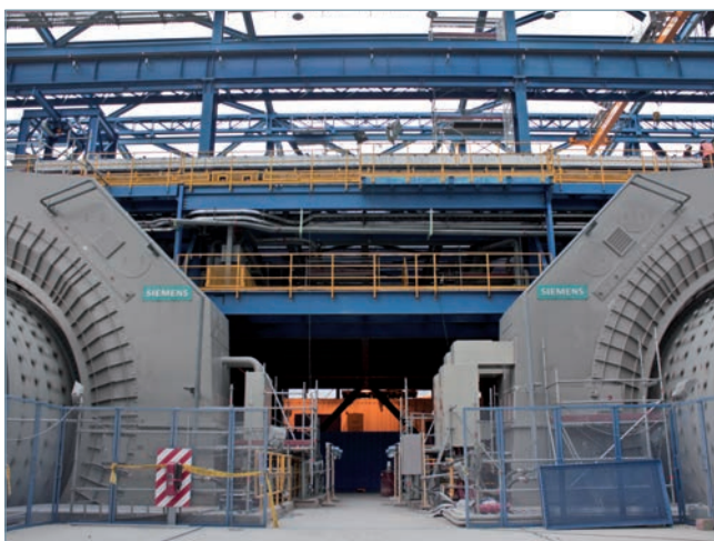
Figure 7 – Both Antapaccay Ball Mills with Gearless Drives of 16,400 kW each
