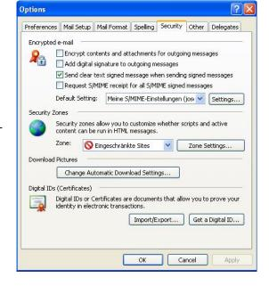
Choose the suggested certificate right next to "Signing Certificate". Then choose a encryption algorithm. Siemens demands "3DES" here. Close everything with "OK". If "3DES" is not available, it could happen that a weaker encryption method will be used. In this case the email cannot be read by Siemens employees. To solve this problem, please contact your Siemens partner and refer to the corresponding manual for Siemens employees.
