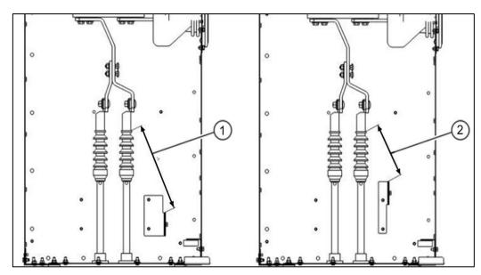
Fig. 214: Minimum distances between cable lug and shielding cover:
