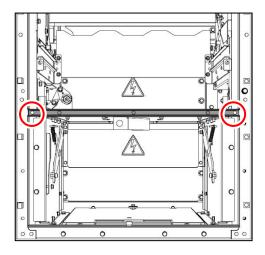
Fig. 262: 2 bolted joints at the labyrinth, front
