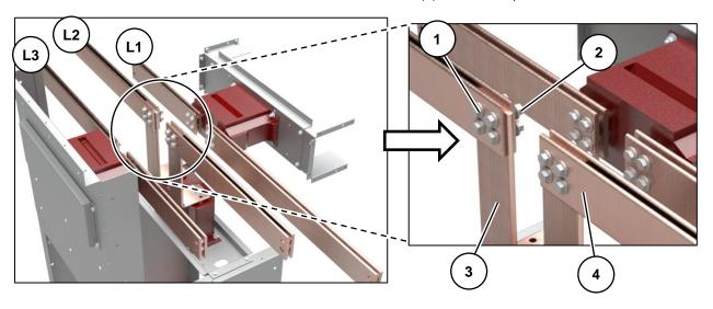
Fig. 63: Busbar current metering panel: Busbar assembly phase L2 (for example, 2500 A busbar)
