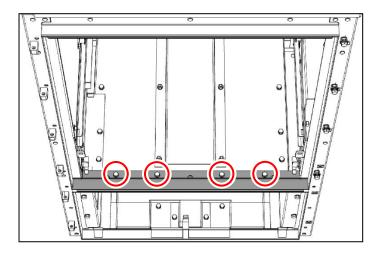
Fig. 171: 4 bolted joints at the labyrinth, top side
