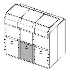
Fig. 265: All panel versions except for contactor panels with panel width 435 mm: Rear wall, 3-panel arrangement
