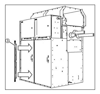
Fig. 85: Panel connection link
