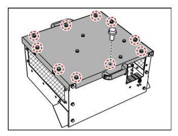
Fig. 113: Fan box connecting bolts (top)
