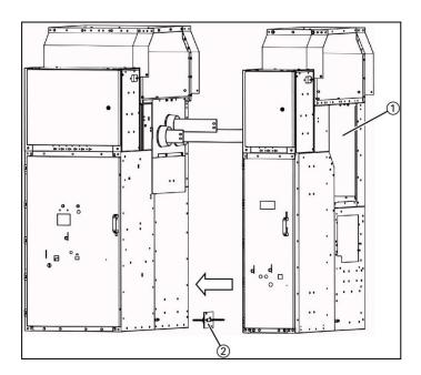
Fig. 84: Connecting element for lining up a contactor panel with panel width 435 mm with a panel featuring a panel width ≥ 600 mm
