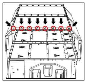
Fig. 90: Bolted joints in the upper area of the PRC
