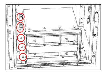
Fig. 240: 6 lateral bolted joints on partition and base frame
