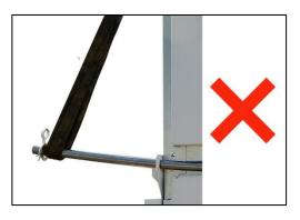
Fig. 38: Heavy weight sling attached incorrectly
