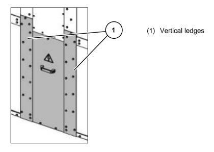
Fig. 190: Contactor panels with panel width 435 mm only: 30 bolts in the ledges
