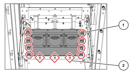
Fig. 250: 11 bolted joints on bushing plate
