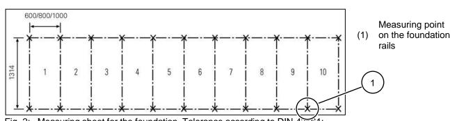
Fig. 2: Measuring sheet for the foundation. Tolerance according to DIN 43061: Straightness 1 mm/1 m length, 2 mm for the total length; evenness 1 mm within 1 m measured length; NXAIR version with I<sub>k</sub> ≤ 31.5 kA and busbar version up to 2500 A (with contactor panels with panel width 600 mm or without contactor panels)
