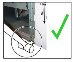
Fig. 25: Permissible application on the right below the switchgear frame
