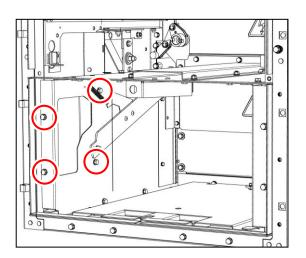
Fig. 173: 4 bolted joints on metal cover in voltage transformer compartment
