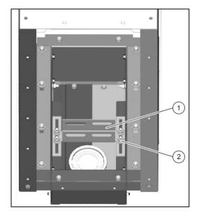
Fig. 219: Assembly of the cable brackets
