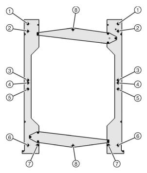
Fig. 17: Drilling template, arrangement for 1000 mm panel width as an example
