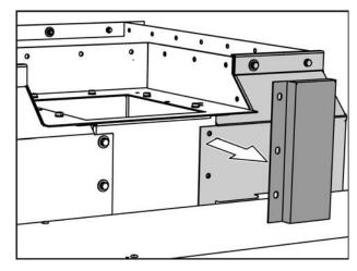
Fig. 110: Front cover at pressure relief duct
