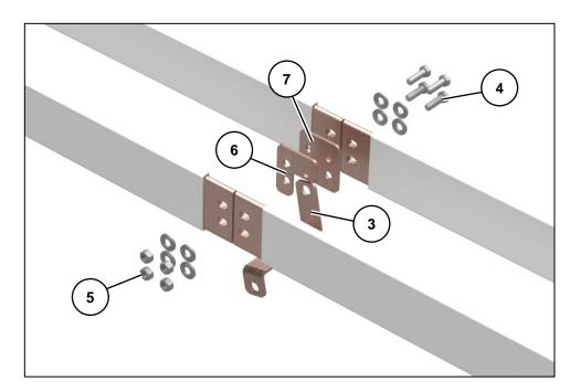
Fig. 75: Detail view of the feeder bar connection (L1 phase as an example)
