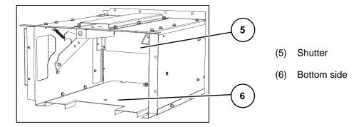
Fig. 254: Voltage transformer compartment
