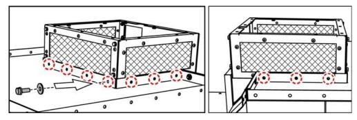
Fig. 117: Fan box connections (laterally)
