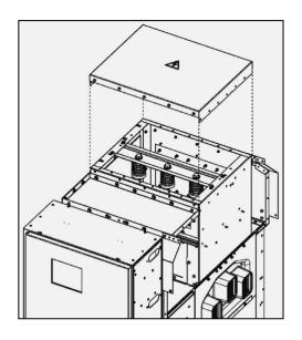
Fig. 97: PRD with e.g. busbar earthing switch installation
