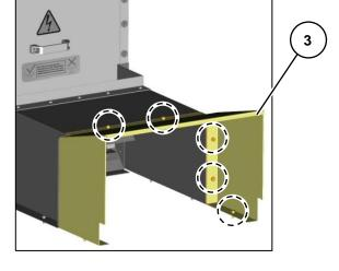
Fig. 164: Front part of ventilation duct, seen from center-right
