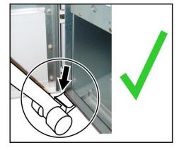
Fig. 26: Permissible application on the left below the switchgear frame
