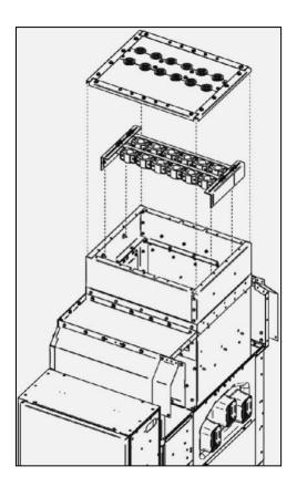
Fig. 98: PRD with cable connection from above
