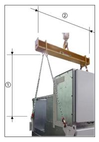
Fig. 40: Transport unit suspended from a crane cross-member
