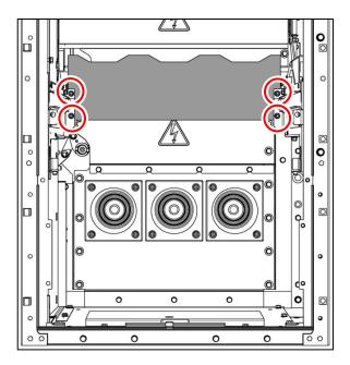
Fig. 179: 4 bolted joints on protection plate of switching-device compartment
