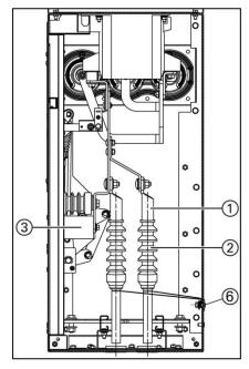
Fig. 208: Rear view of connection compartment in contactor panel
