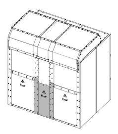
Fig. 186: Contactor panels with panel width 435 mm only:
