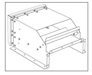
Fig. 154: Ventilation duct removed
