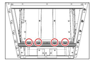
Fig. 263: 4 bolted joints at the labyrinth, top side
