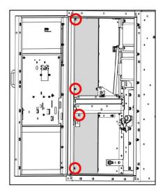
Fig. 88: Fastening the wiring duct covers
