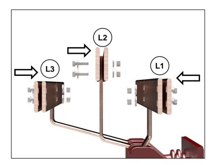
Fig. 54: Side view of 2000 A / 2500 A busbar assembly, feeder  $\leq$  1250 A,  $U_r \leq$  12 kV,  $I_k \leq$  31.5 kA or feeder  $\leq$  2500 A,  $I_k \leq$  40 kA with forced ventilation
