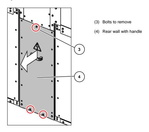
Fig. 192: Contactor panels with panel width 435 mm only: Removing the rear wall
