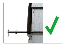
Fig. 37: Heavy weight sling attached correctly
