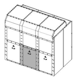
Fig. 185: All panel versions except for contactor panels with panel width 435 mm and switch-disconnector panel: Rear wall, 3-panel arrangement
