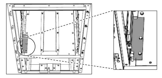
Fig. 172: 3 bolted joints on wiring duct cover
