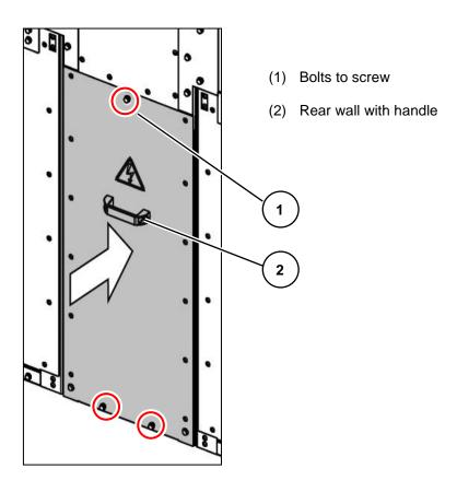
Fig. 269: Contactor panels with panel width 435 mm only: Installing and fixing the rear wall
