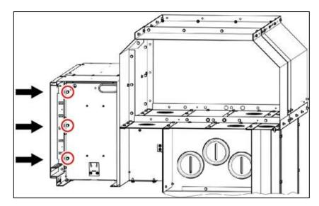
Fig. 91: Bolted joints at the low-voltage compartment
