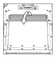
Fig. 148: Folding the air guide upwards
