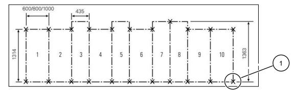
Fig. 3: Measuring sheet for the foundation. Tolerance according to DIN 43661: Straightness 1 mm/1 m length, 2 mm for the total length; evenness 1 mm within 1 m measured length; NXAIR version with  $I_k \le 31.5$  kA and busbar version up to 2500 A (with contactor panels with panel width 435 mm)
