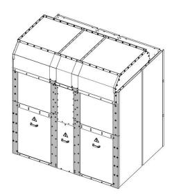
Fig. 93: Contactor panel with panel width 435 mm (center): Panel connection links and bolted joints at the rear
