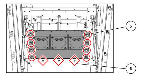
Fig. 182: 11 bolted joints on bushing plate
