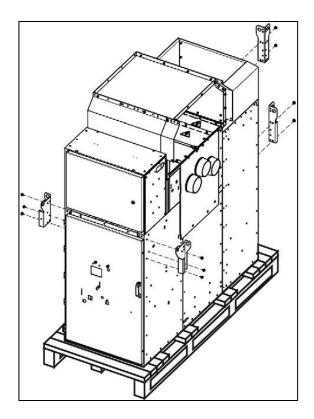
Fig. 31: Example for a panel with rear duct:
