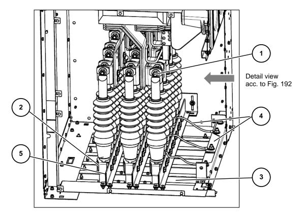
Fig. 205: Connection compartment with connections for 6 cables per phase (example)
