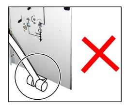
Fig. 28: Incorrect application of lifting tool
