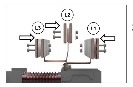
Arrowhead indicates the inserting direction of the bolts
