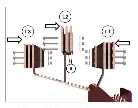
Fig. 58: Side view of 3150 A / 4000 A busbar assembly, feeder  $\leq$  1250 A, Ur  $\leq$  12 kV
