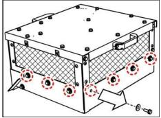
Fig. 112: Fan box connecting bolts (laterally)
