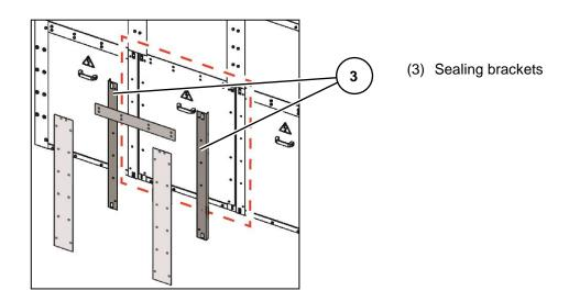
Fig. 188: All panel versions except for contactor panels with panel width 435 mm and switch-disconnector panel: Removing the sealing brackets
