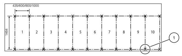
Fig. 4: Measuring sheet for the foundation. Tolerance according to DIN 43661: Straightness 1 mm/1 m length, 2 mm for the total length; evenness 1 mm within 1 m measured length; NXAIR version with  $I_k \leq 31.5$  kA and busbar version up to 3150/4000 A) and NXAIR version with  $I_k = 40$  kA (with or without contactor panels)
