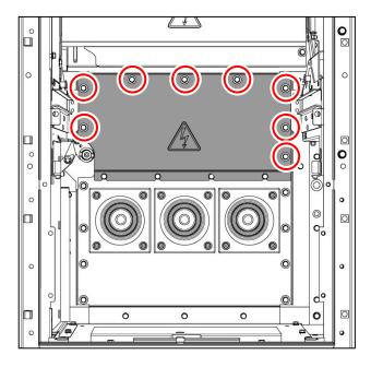
Fig. 180: 8 bolted joints on partition
