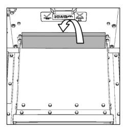
Fig. 242: Folding the air guide downwards
