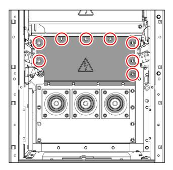
Fig. 252: 8 bolted joints on partition
