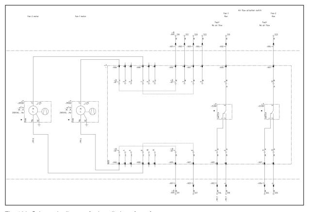
Fig. 120: Schematic diagram for installation of two fans
