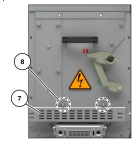
Fig. 230: 2 bolted joints on the heater
