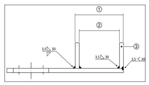
Fig. 14: Side view of the fixing plate
