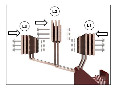
Fig. 60: Side view of 3150 A / 4000 A busbar assembly, feeder 2500 A,  $U_r \le 12$  kV,  $I_k \le 31.5$  kA or feeder 2500 A,  $I_k \le 40$  kA with forced ventilation
