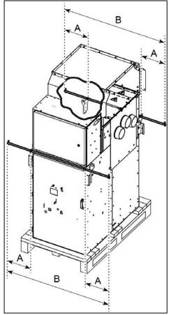
Fig. 35: Crane rods at the front and rear
