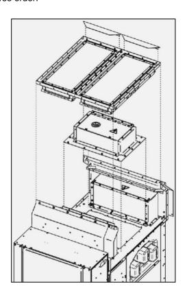
Fig. 95: PRD with natural ventilation
