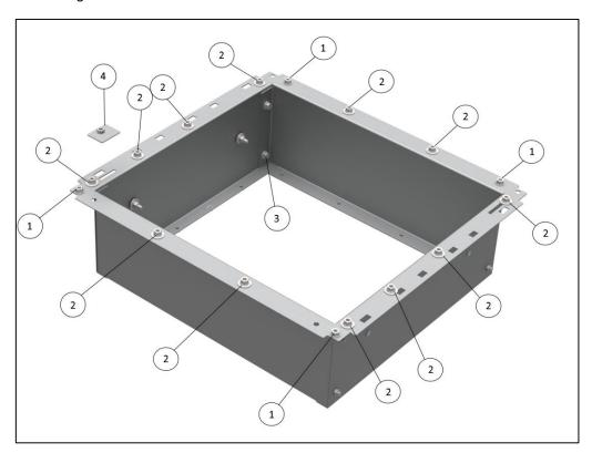
Fig. 211: Assembly of the front and side plates
