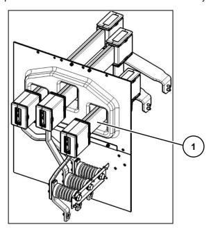
Fig. 70: Contactor panels with panel width 435 mm:
