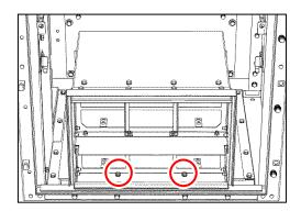
Fig. 152: 2 bolted joints on base frame at the front
