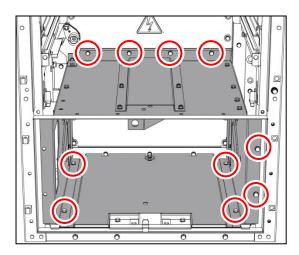
Fig. 176: 10 bolted joints at voltage transformer compartment
