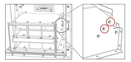
Fig. 243: Bolts for fixing the holder
