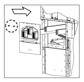
Fig. 81: Mounting the transverse partition plate from the left on the switch-disconnector panel
