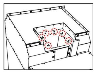
Fig. 109: Pressure relief duct for fan box
