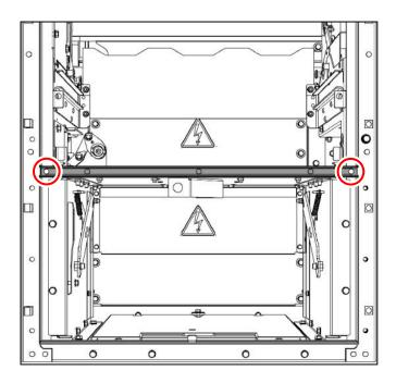
Fig. 170: 2 bolted joints at the labyrinth, front
