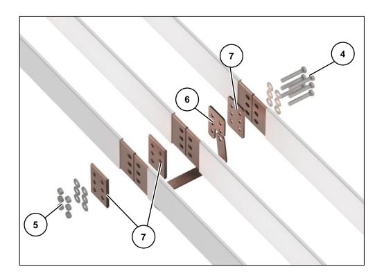
Fig. 78: Detail view of the feeder bar connection (L1 phase as an example)
