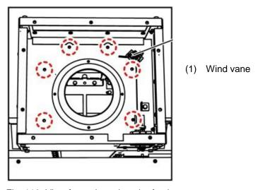
Fig. 116: View from above into the fan box
