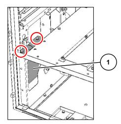
Fig. 174: 2 bolted joints on metal cover in switching-device compartment
