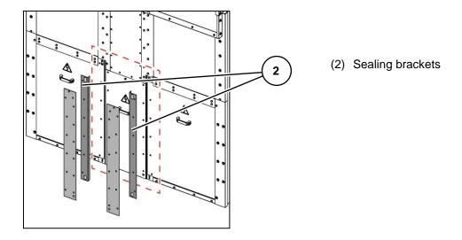
Fig. 191: Contactor panels with panel width 435 mm only: Removing the sealing brackets
