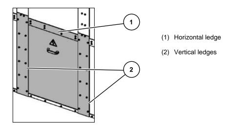
Fig. 187: All panel versions except for contactor panels with panel width 435 mm and switch-disconnector panel: 36 bolts on ledges
