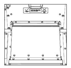
Fig. 149: Air guide folded upwards
