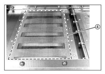
Fig. 103: View onto the ventilation system in the pressure relief duct
