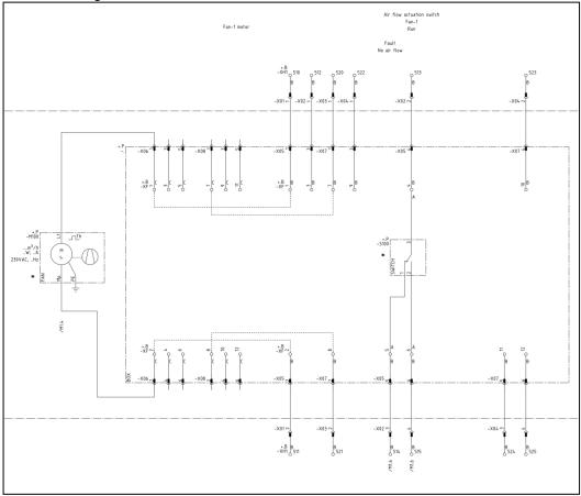
Fig. 119: Schematic diagram for installation of one fan
