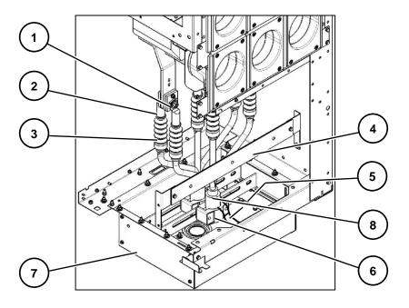
Fig. 209: Side view of connection compartment with three-core cables
