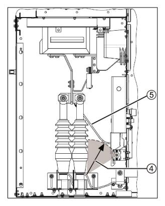
Fig. 201: Connection compartment on panel with removable voltage transformers:  $U_r = 17.5 \text{ kV}$
