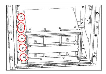
Fig. 151: 6 lateral bolted joints on partition and base frame
