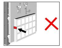
Fig. 275: Ventilation flap **not** in operational position, negative indication
