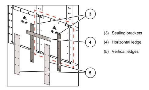
Fig. 268: All panel versions except for contactor panels with panel width 435 mm: Installing the sealing brackets and ledges
