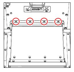
Fig. 150: 4 bolted joints on partition
