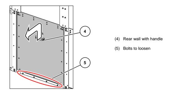
Fig. 189: All panel versions except for contactor panels with panel width 435 mm and switch-disconnector panel: Removing the rear wall
