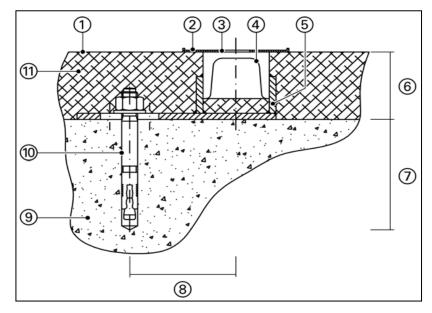
Fig. 13: Bolted floor fixing
