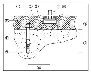
Fig. 7: Bolted floor fixing
