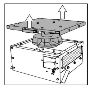
Fig. 114: Fan box roof plate
