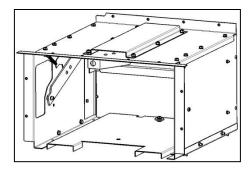
Fig. 178: Voltage transformer compartment, removed
