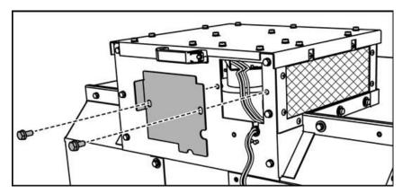
Fig. 124: Assembling the cover
