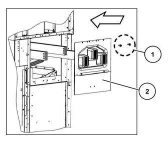
Fig. 82: Mounting the transverse partition plate from the right on the switch-disconnector panel
