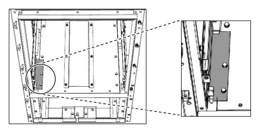
Fig. 259: 3 bolted joints on wiring duct cover
