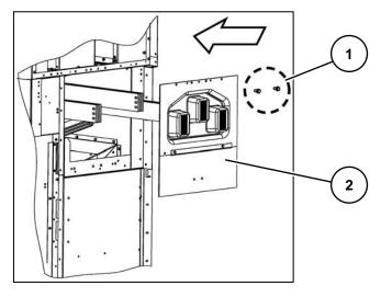
Fig. 67: Mounting the transverse partition plate from the right, panel depth 1500/1540/1650 mm
