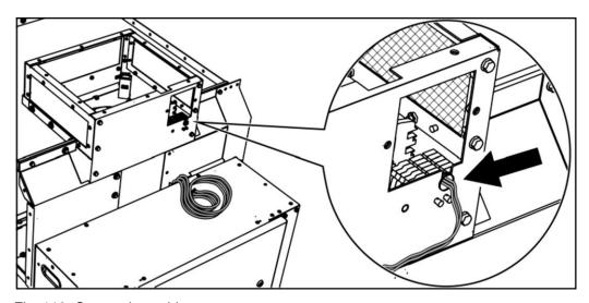
Fig. 118: Connection cables
