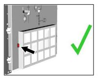
Fig. 274: Ventilation flap in operational position, positive indication
