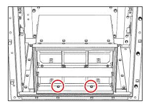
Fig. 239: 2 bolted joints on base frame at the front
