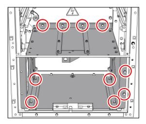
Fig. 255: 10 bolted joints at voltage transformer compartment
