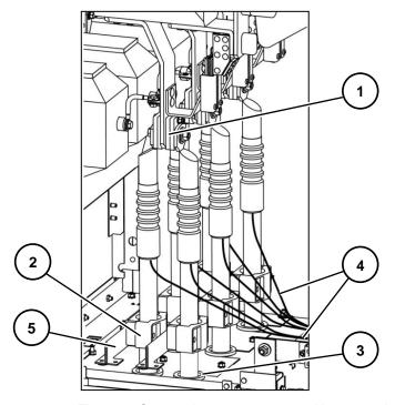
Fig. 204: Connection compartment with connections for 2 cables per phase (example)
