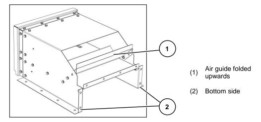
Fig. 237: Ventilation duct with air guide folded upwards
