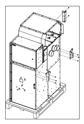
Fig. 30: Example for a panel with end wall: 3 craning angles with 3 or 2 bolted joints M8x20 each
