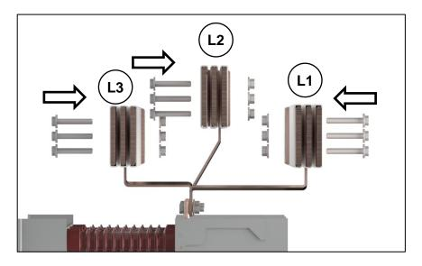
Fig. 79: Side view of 3150 A / 4000 A busbar assembly, feeder 1250A
