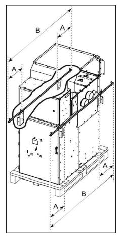
Fig. 36: Crane rods at the side
