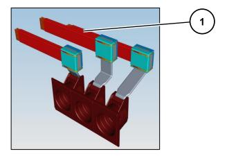
Fig. 68: Detail view of busbar system with plastic tubes; right end panel as an example
