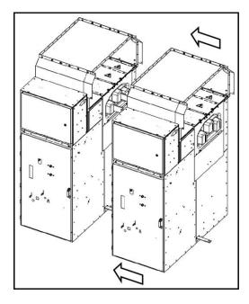
Fig. 83: Aligning the panel
