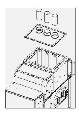
Fig. 99: PRD with bar connection from above
