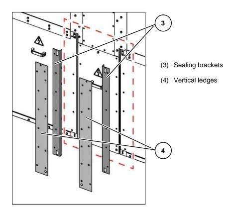
Fig. 270: Contactor panels with panel width 435 mm only: Installing the sealing brackets and ledges
