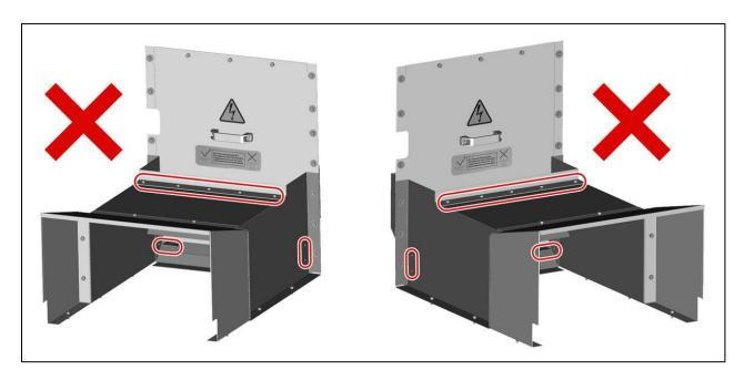
Fig. 161: Bolted joints not to be loosened
