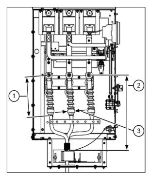
Fig. 202: Dimensions of three-core cables (except for contactor panel with panel width 435 mm)
