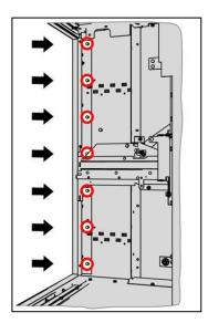
Fig. 87: Bolted joints in the switching-device compartment
