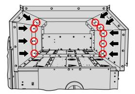
Fig. 89: Bolted joints inside the PRC
