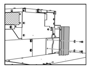
Fig. 125: Installing the front cover
