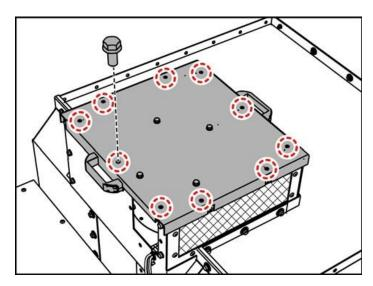
Fig. 122: Fixing the roof plate
