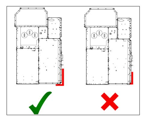
Fig. 43: Permissible application on the switchgear frame
