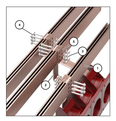
Fig. 57: Assembly of 3150 A / 4000 A busbar, feeder  $\leq$  1250 A,  $U_r \leq$  12 kV
