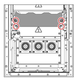
Fig. 253: 4 bolted joints on protection plate of switching-device compartment
