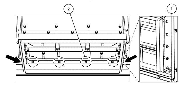
Fig. 46: 6 bolted joints to be removed from the ventilation duct
