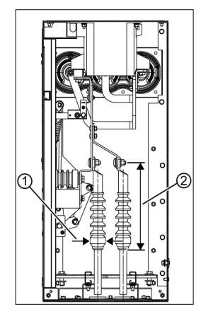
Fig. 199: Dimensions of single-core cables in contactor panel with panel width 435 mm (rear view)
