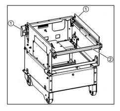
Fig. 44: Service truck with transport protection
