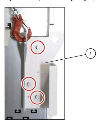
Fig. 32: Craning angle (1) mounted at the side of the panel front (3 bolted joints), shown here with crane hooks
