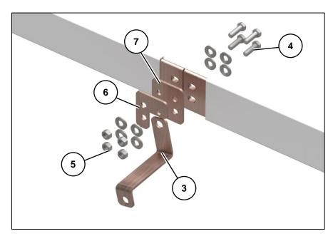
Fig. 72: Detail view of the feeder bar connection (L1 phase as an example)
