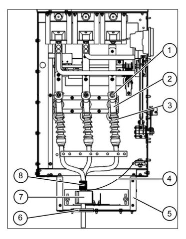
Fig. 215: Side view of connection compartment with three-core cables in contactor panel with panel width 435 mm
