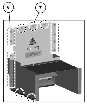
Fig. 167: Ventilation duct and partition, seen from center-right
