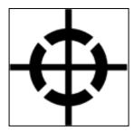
Fig. 20: Symbol for center of gravity
