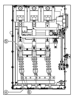
Fig. 207: Side view of connection compartment in contactor panel
