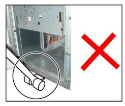
Fig. 27: Incorrect application of lifting tool
