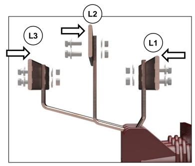
Fig. 52: Side view of 1250 A busbar assembly, feeder  $\leq$  1250 A,  $U_r \leq$  12 kV
