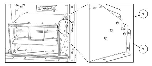
Fig. 147: Bolts for detaching the holder
