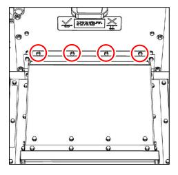
Fig. 241: 4 bolted joints on partition
