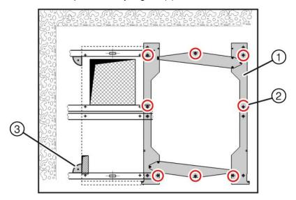
Fig. 18: Applied drilling template, arrangement for 1000 mm panel width as an example
