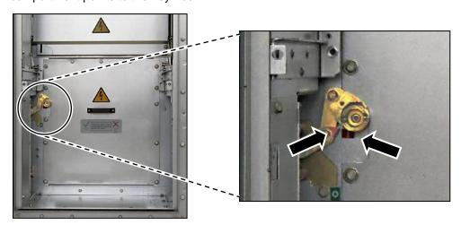
Fig. 132: All panel versions except for contactor panels with panel width 435 mm and switchdisconnector panels: Additional position indicator of feeder earthing switch in switching-device compartment
