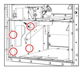
Fig. 256: 4 bolted joints on metal cover in voltage transformer compartment
