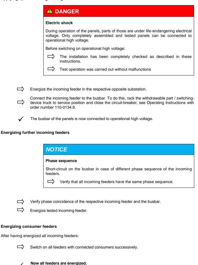
Thus, the switchgear is completely in operation.
