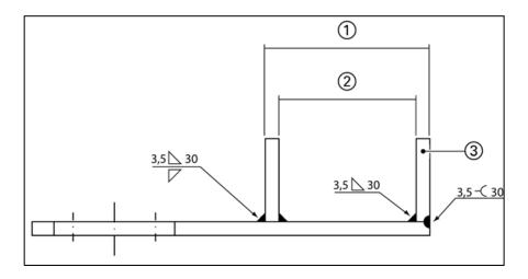
Fig. 10: Side view of the fixing plate
