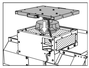
Fig. 121: Installing the roof plate
