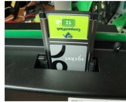
10. Reinstall the A80407 Display Module in the GCP 4000. After completion of the boot process the following message will appear: "Creating file description data. DT will restart when done" (see figure #13). Select **OK** to initiate the process.
