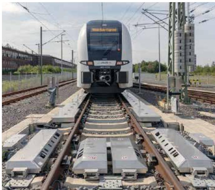
Predict and prevent: an RRX multiple-unit enters the automatic vehicle identification and measurement (AVI) system at the fully digitised depot of Siemens Mobility Customer Services in Dortmund, Germany.
