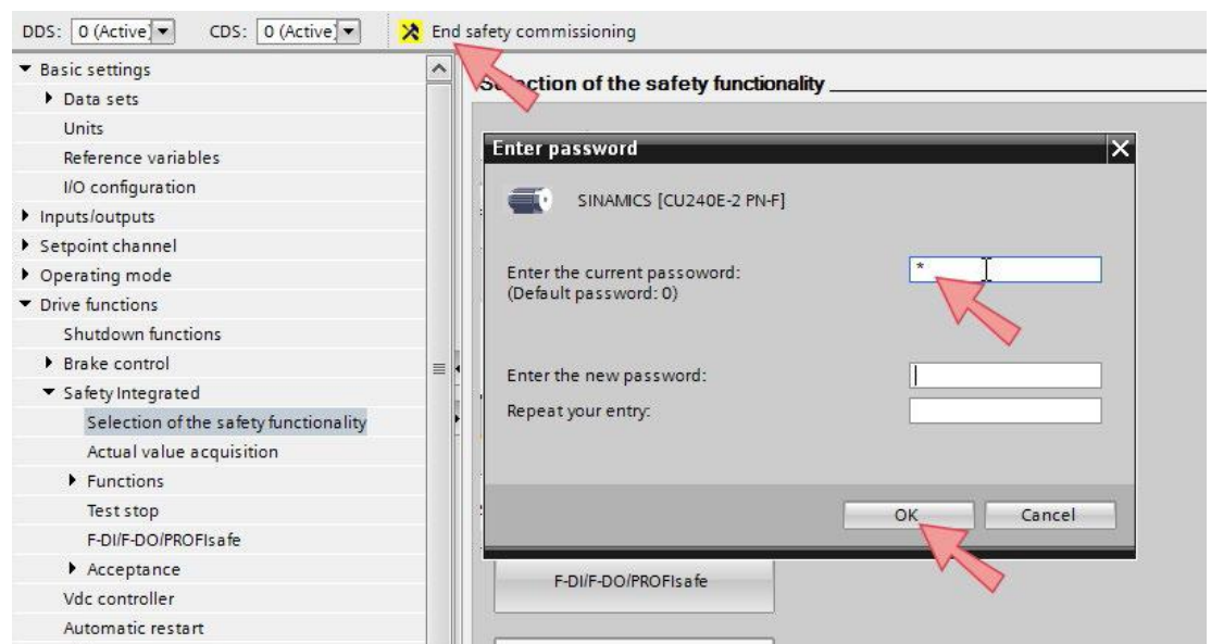
Figure 9-17 Activating Safety Integrated in the drive
