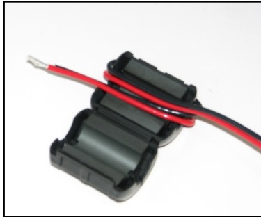
Figure 2-5 EMI Filter Installation (Showing Wire Loops)
