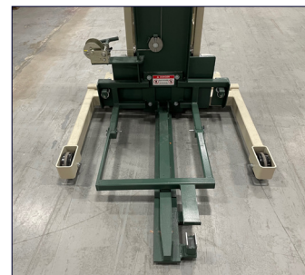
Figure 49: Lift truck forks with auxiliary tray adapter
