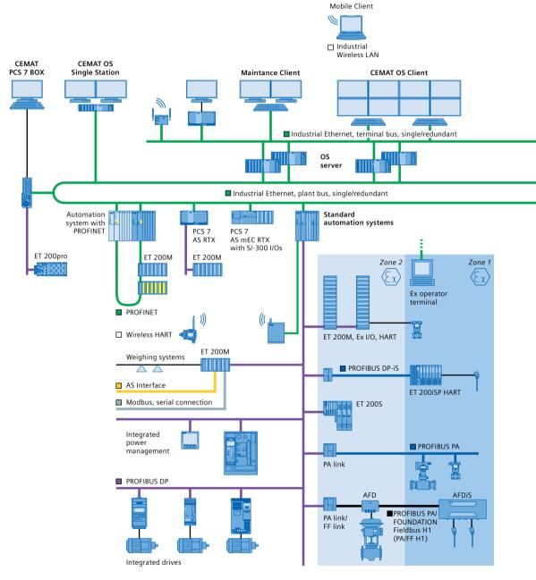
The entire hardware structure of the process control system is hierarchically displayed at the maintenance station.
