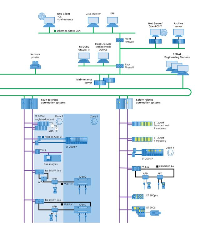
With SIMATIC PCS 7 and CEMAT, all components that can be diagnosed – like the PCs, bus components, automation systems, and the entire decentralized periphery such as I/O modules and intelligent field devices – are integrated with Asset Management.
