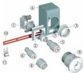
Fig. 3.1.6 – DIAZED® system components
