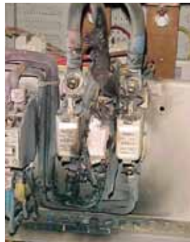
Fig. 5.8.1 – Unsuccessful disconnection of current resonance
