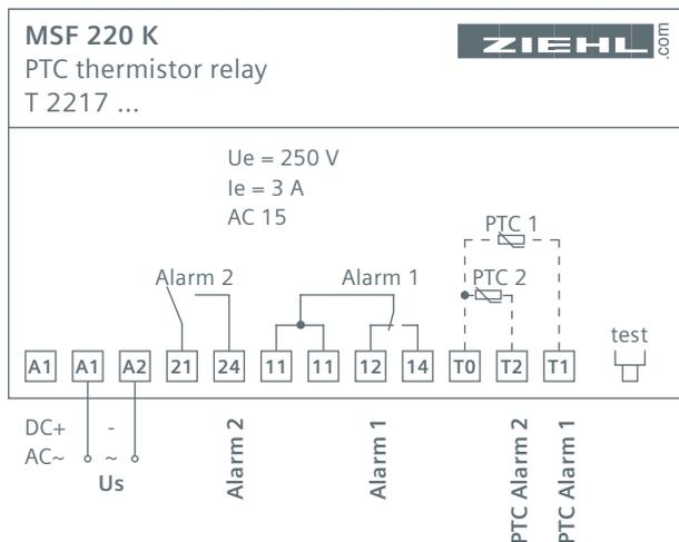
Fig. 6: Connecting diagram of a power supply for the tripping unit for PTC sensors
