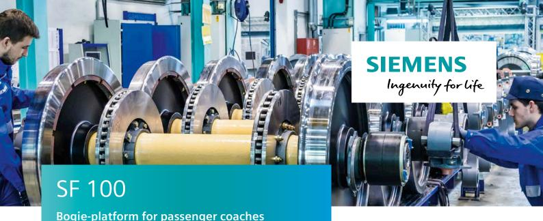
The bogie-platform SF 100 is a further development of the bogie-family SF 400. The SF 100 was designed for push-pull service in locomotive-hauled passenger coaches and for trailer-bogies in multiple units. The maximum operational speed is 249 km/h.
