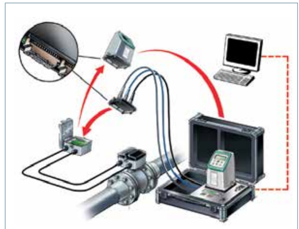
Verificator connection on the SITRANS F M flowmeter
