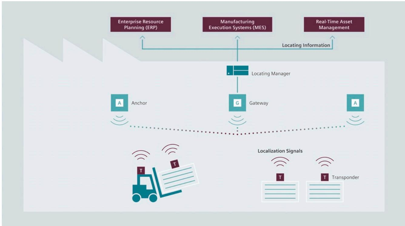
The infrastructure of SIMATIC RTLS can be used for a wide variety of applications.
