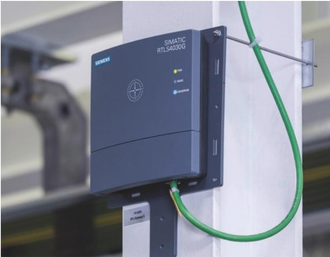
Anchors and Gateways provide the “where” of all mobile objects – from manufacturing equipment to materials and components to the finished product.
