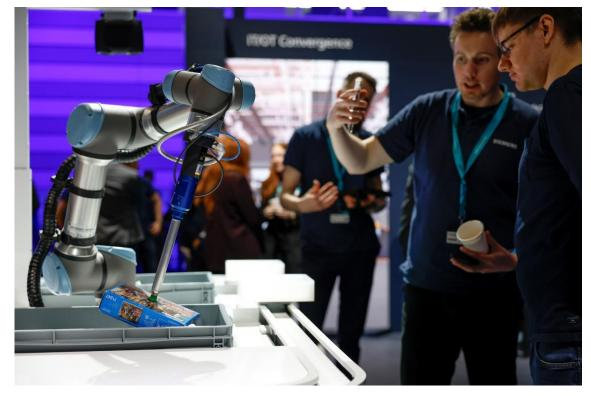
With Simatic Robot Pick AI Pro, an industrial vision AI for the development of AI-supported picking robots, Siemens demonstrates in a highlight showcase how the combination of software-defined and data-driven automation creates more adaptability and flexibility in automation solutions.
