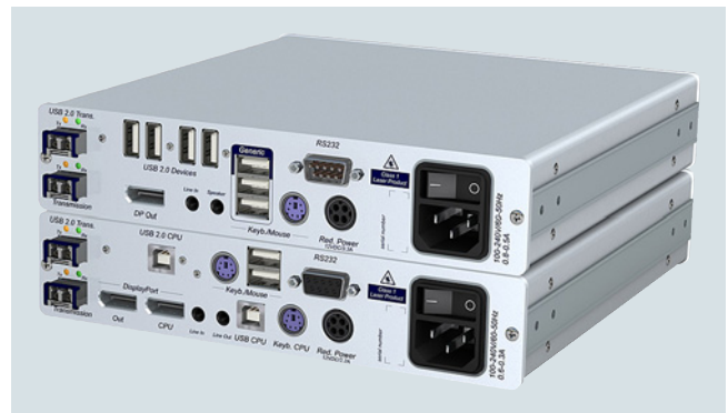
KVM Extender DP1.2-Vision, transmitter (bottom) and receiver (top)
