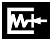
Fig. 2: Indication: "Spring charged"
