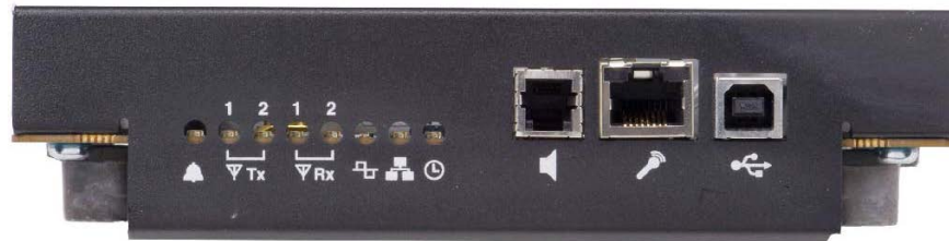
Figure 8-5 Station Control Module (Front View)
