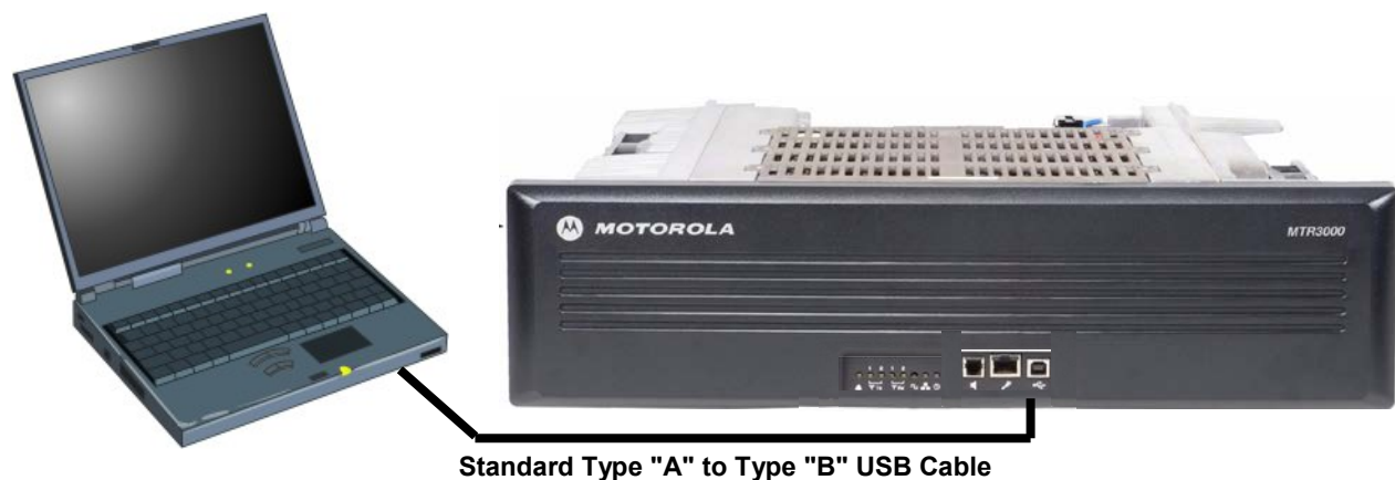
Figure 6-30 PC to MTR3000 Connection
