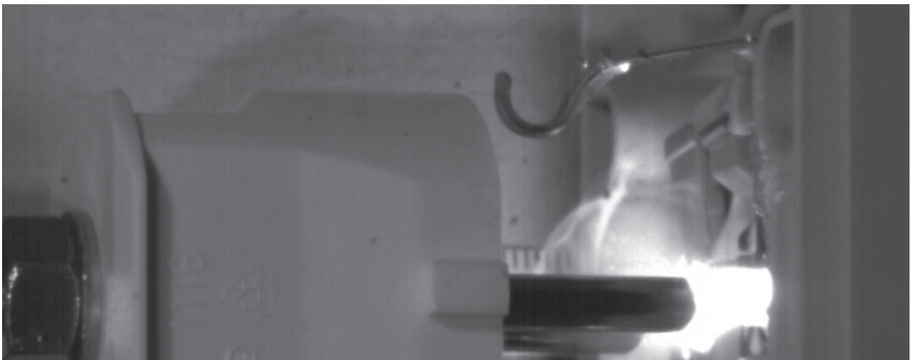
Fig. 9: Arcing when a live plug (exposed to direct current) is pulled [12]
