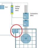
Non-contact protective door monitoring with 3SE63 RFID switch
