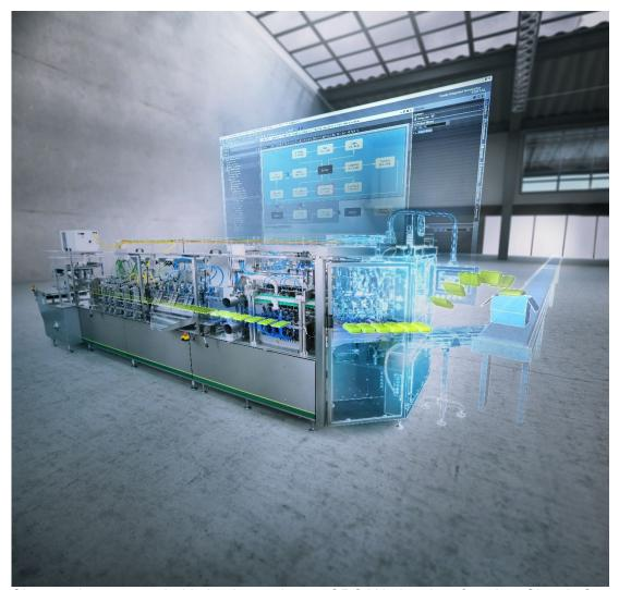
Siemens has succeeded in implementing an OPC UA data interface in a Simatic S7-1500 controller according to a companion specification using the OMAC PackML (Packaging Machine Language). This makes it easier for end customers and line integrators to integrate packaging machines and connect them to line or MES systems.
