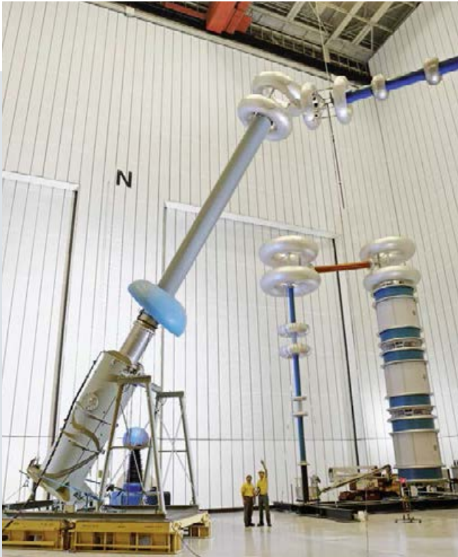
Fig. 77: Transformer bushing – 800 kV UHVDC – project Yunnan-Guangdong, China
