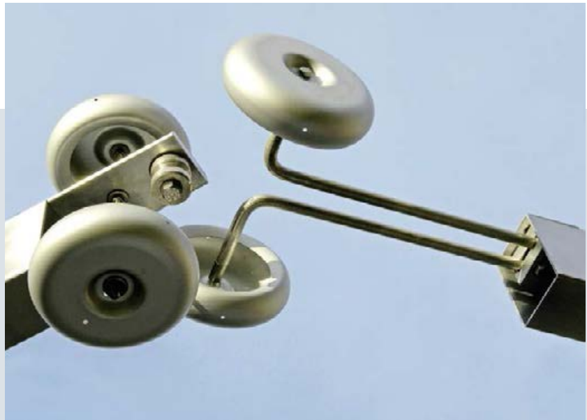
Fig. 25: Block and finger contact system
