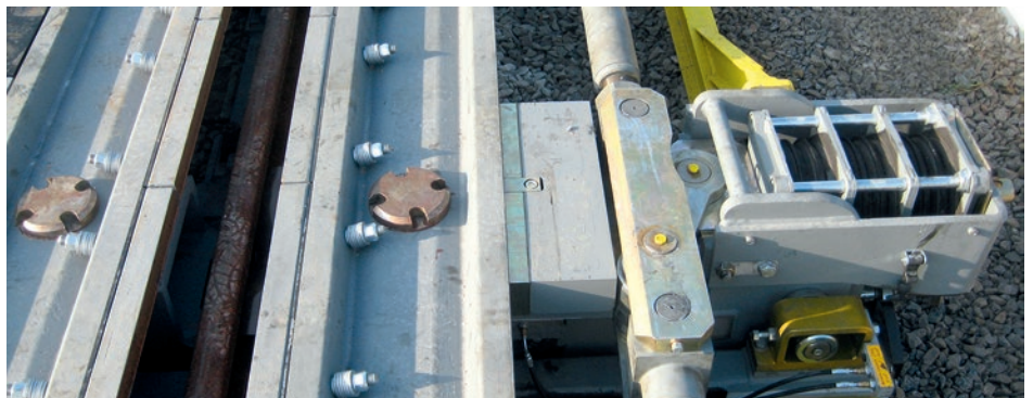
Retarding principle with rubber-spring assemblies
