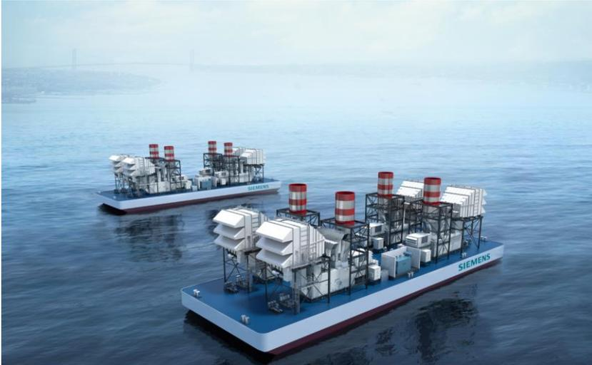
The picture shows two SeaFloat power barges each equipped with four SGT-A65 gas turbines.
