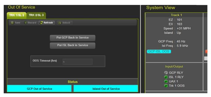
Figure 4-6: Island Out of Service Indications on WebUI
