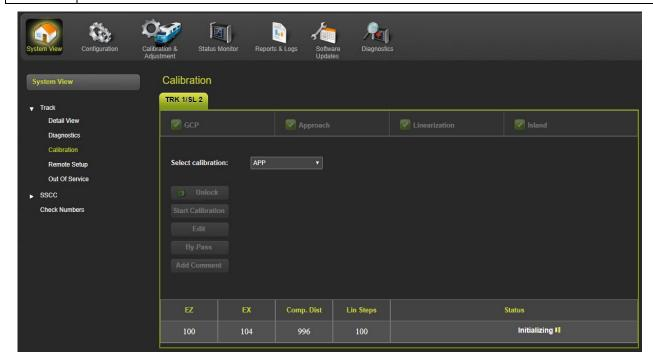
Figure 7-7: Calibration Initializaing
