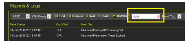
Figure 3-22 WebUI: Event Log Text Filter
