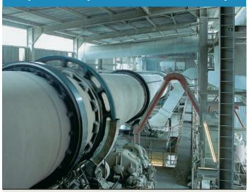
The main technology of a cement plant is the rotary kiln. This is the sector with the highest investment costs and the largest energy requirements. The optimum range of a rotary kiln with regard to the use of fuel is extremely limited. It is defined by the concentrations of oxygen and carbon monoxide.
