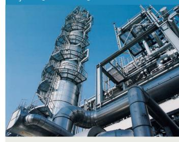
Flue gas denitrification is divided into primary and secondary measures. Primary measures are carried out directly on the burner. Secondary measures are based on chemical reactions between the flue gas and an additionally introduced reagent.
