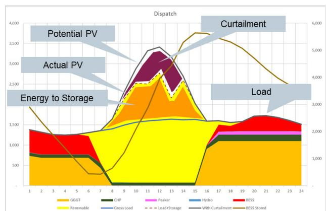
Figure 2: Timing of energy storage charging curtailment impacts
