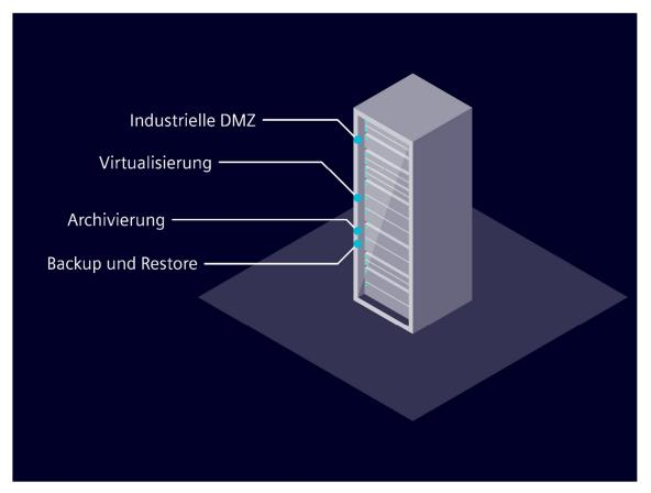
Image source Siemens: Structure of the Siemens Industrial Automation DataCenter (IADC)
