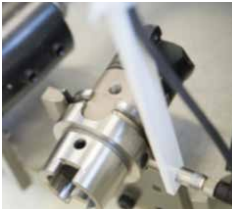
Tool holder with RFID tag in tool changer
