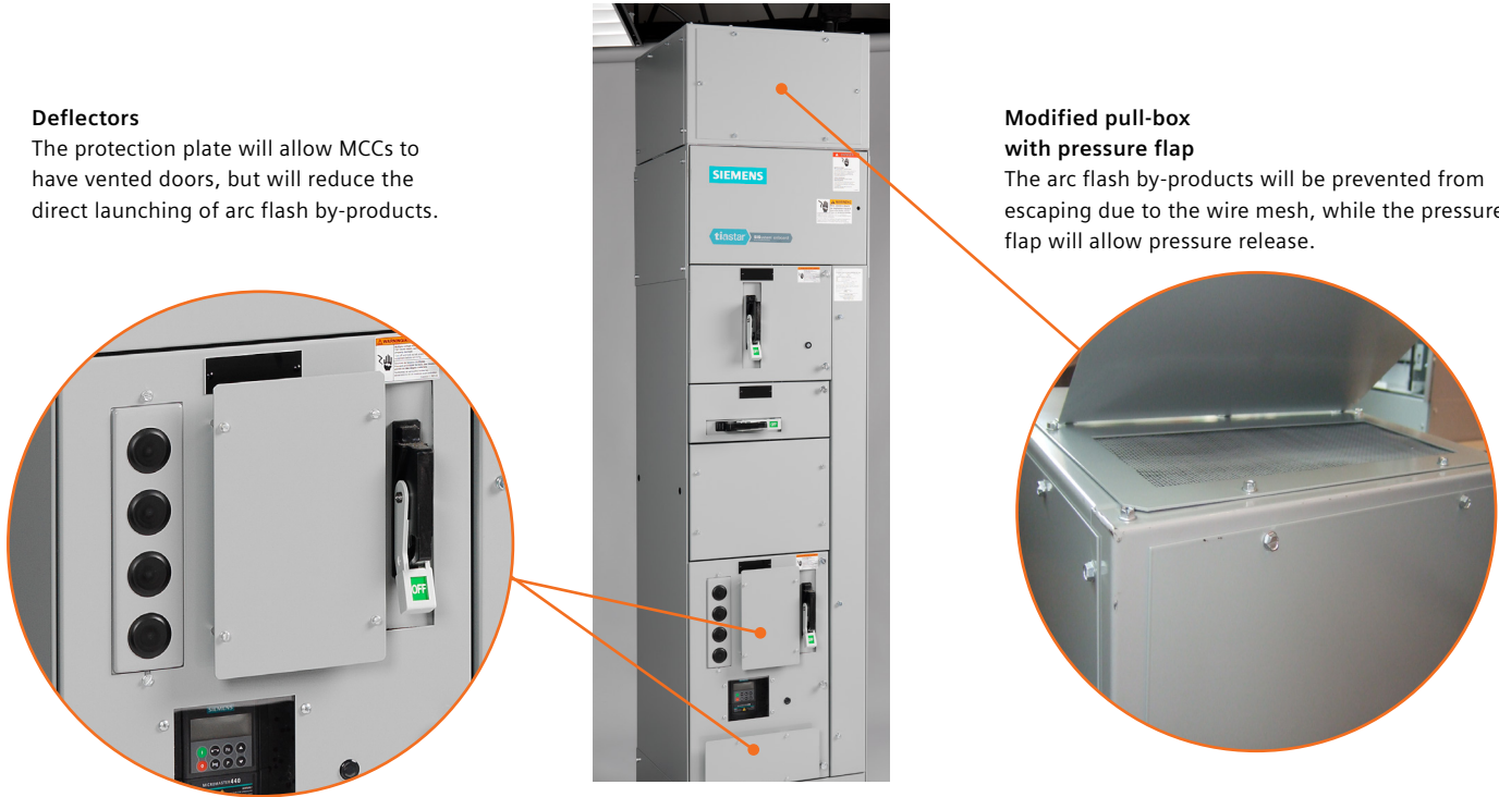
Figure 2: Closed door view - Arc Resistant MCC
