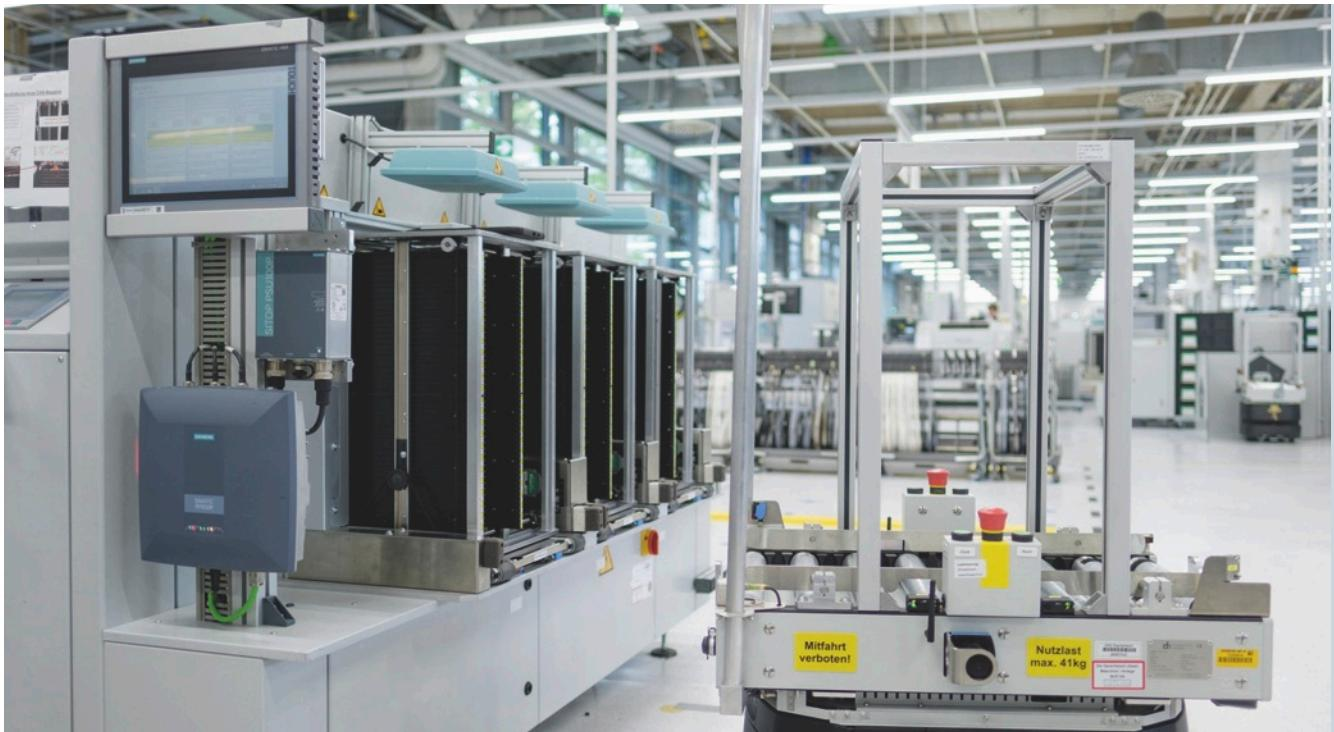
At the Siemens plant in Karlsruhe, automated guided vehicles (AGVs) are replacing the rigid linking with materials handling technology.
