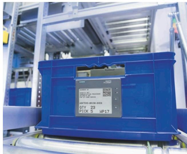
The transponders with ePaper display from SIMATIC RTLS enable novel interactions between man and machine.
