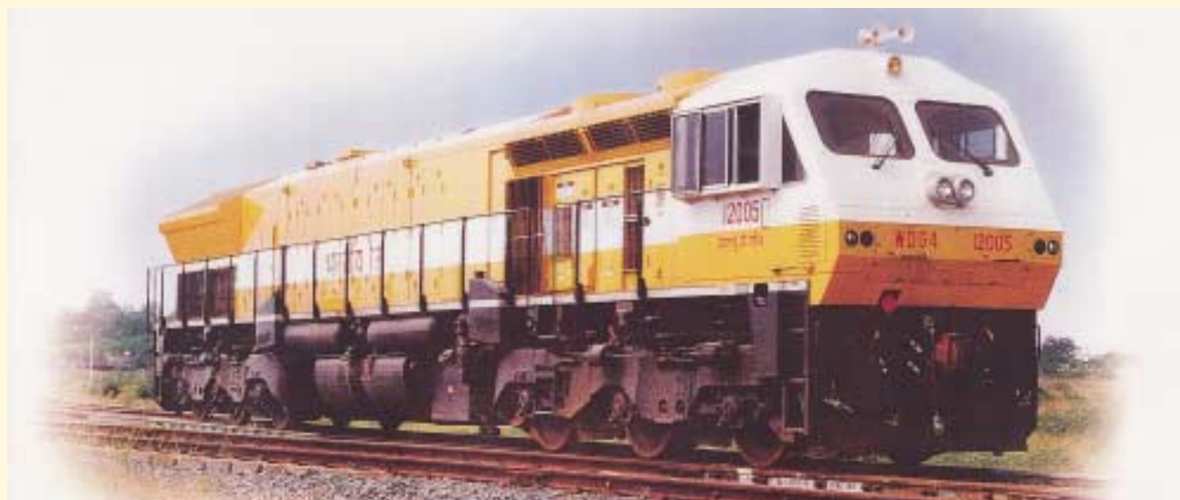
Indian Railway's first three-phase 4000 HP diesel electric loco with traction electrics from Siemens.
