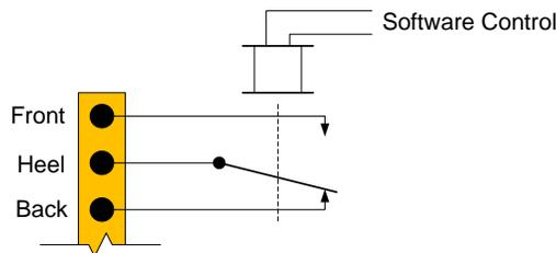
**Figure 3-12: Relay Output Hardware Internals**
