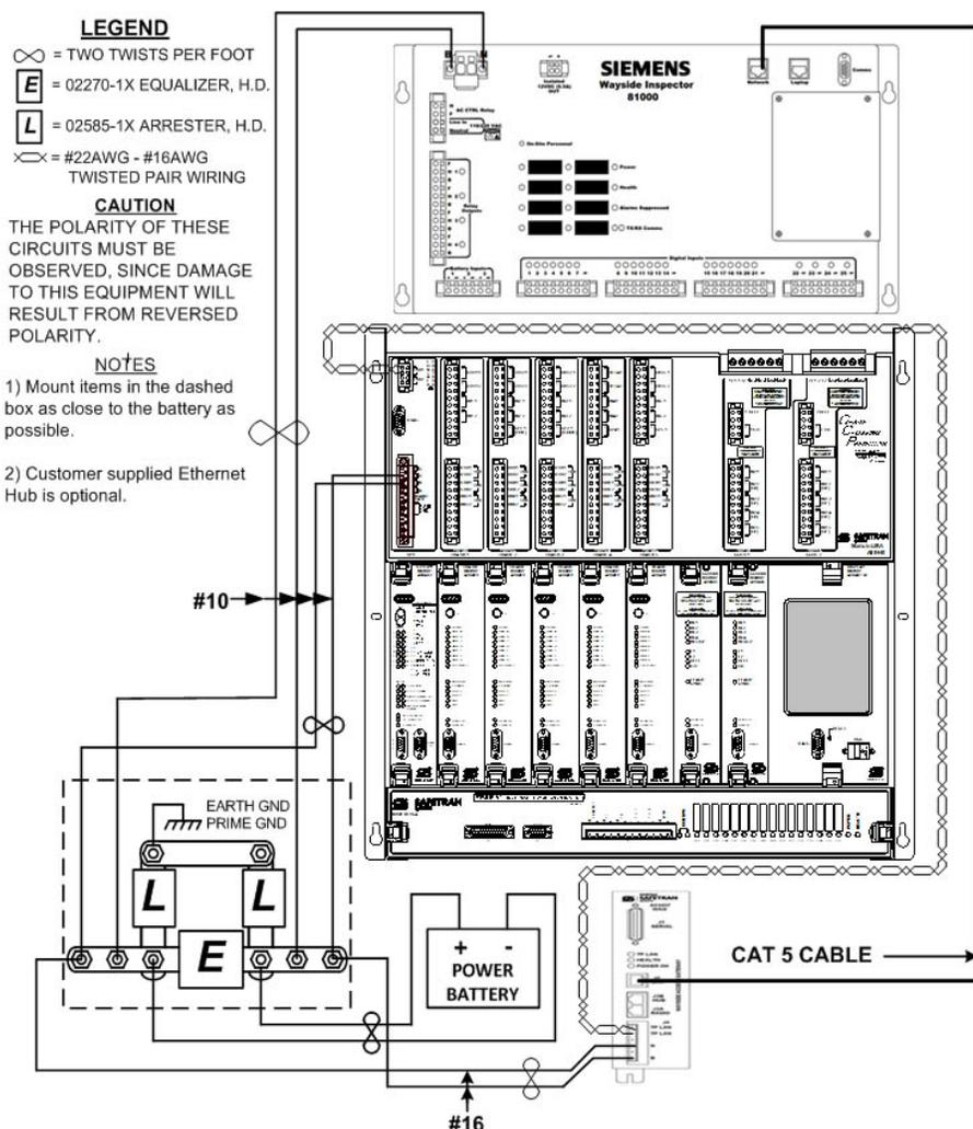
**Figure 6-4: WI Connected to the Model 4000 Grade Crossing Predictor (GCP) via the Wayside Access Gateway (WAG) with WI Configured for Warning Time Inspection**
