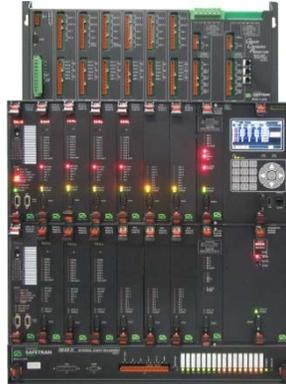
**Figure 4-4: The Model 4000/5000 Grade Crossing Predictor (GCP)**
