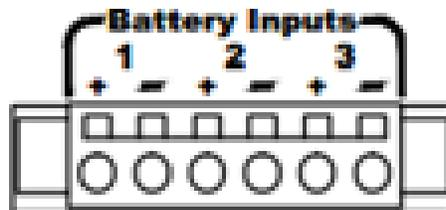
**Figure 3-10: Battery Input Connector**
