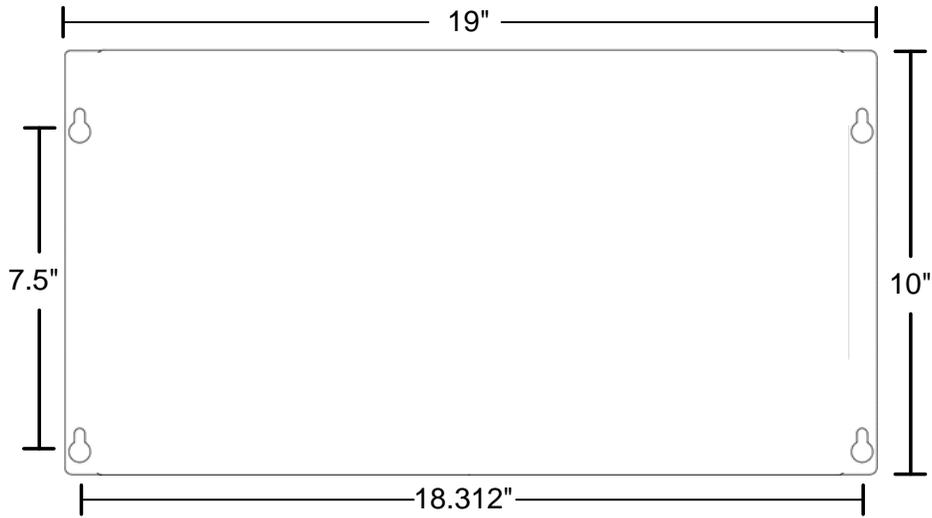
**Figure 3-14: Wayside Inspector Mounting Dimensions**
