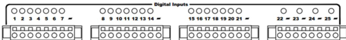
Figure 3-9: Digital Input Connectors and LEDs
