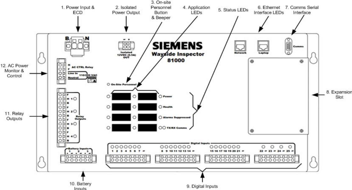
Figure 3-1: The Siemens Wayside Inspector, A81000 Connectors
