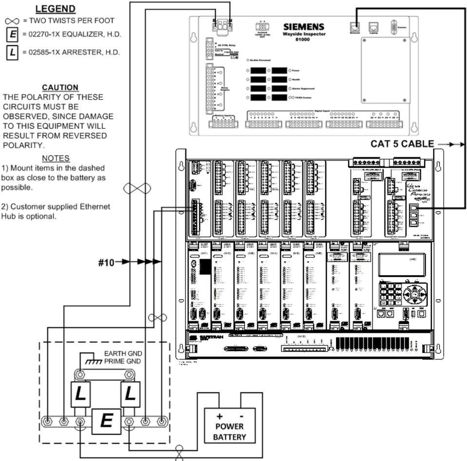
**Figure 6-3: Wayside Inspector Connected to the Model 5000 Grade Crossing Predictor (GCP) with WI Configured for Warning Time Inspection**
