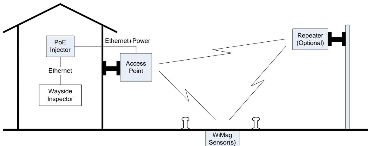
**Figure 4-5: The Wireless Magnetometer (WiMag) Sensor System**
