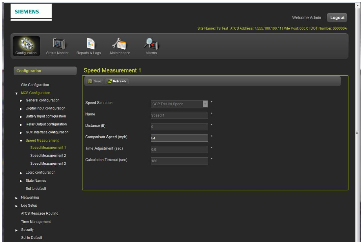
Figure 5-10: The Speed Measurement “N” Screen
