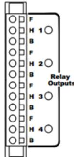
**Figure 3-11: Relay Output Connector and LEDs**
