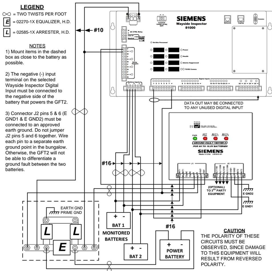
**Figure 6-2: Recommended Wiring for WI Connected to Ground Fault Tester 2 (GFT2) with WI Configured for Grounds Inspection**
