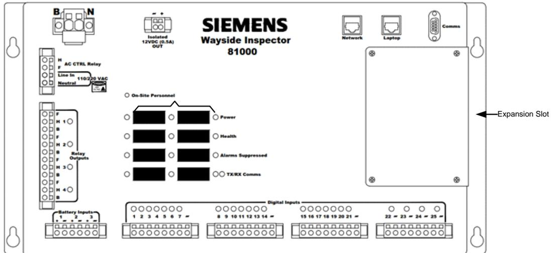
Figure 3-8: Hardware Expansion Slot
