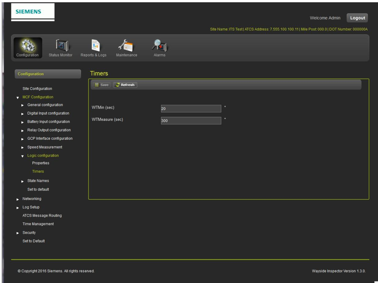
**Figure 5-12: The Logic Configuration Timers Screen**
