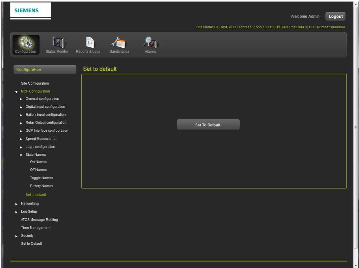
Figure 5-17: The MCF Configuration Set to Default Screen
