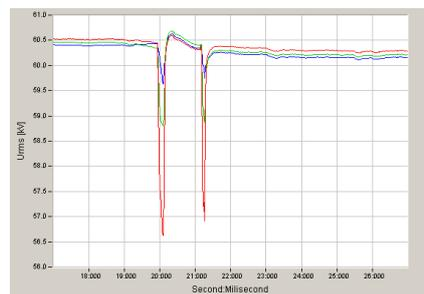
Figure 3: Voltage drops due to faults in the supply grid often result in the failure of variable speed drives (in this example: short interruption after a fault in the high-voltage grid)
