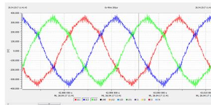
Figure 2: High-frequency oscillations often result in faults in electronic equipment (in this example: voltage in an industrial grid with 100% power converter load – 400 V)
