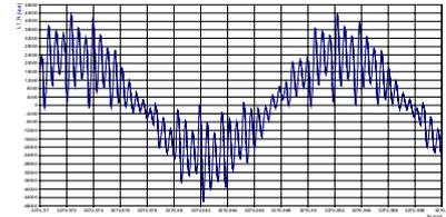
Figure 4: Large distortions in voltages and currents are often caused by resonances in the grid and are often not manifested until the connected equipment is permanently damaged (in this example: voltage in an industrial grid, 34.5 kV)
