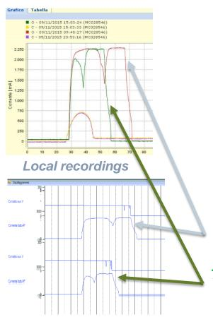
This situation has led the customer to the decision for an intervention of maintenance on condition in order to avoid the repetition of the anomalous event and avoid the risk of a failure (missing of opening operation on command).
